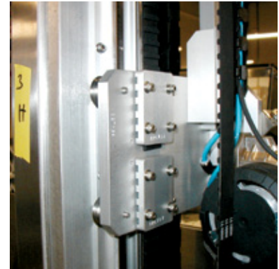
DualVee is used to raise, lower and guide product from one conveyor line to another for this pharmaceutical, cosmetic and personal care packaging machinery.
